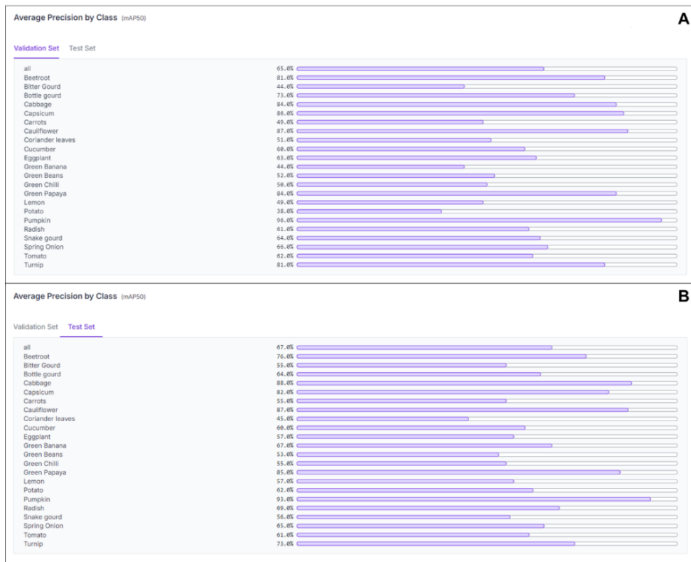
Figure 6. Class-wise average precision of the Roboflow 3.0 Object Detection (Accurate) model on the (A) validation set and (B) test set.
